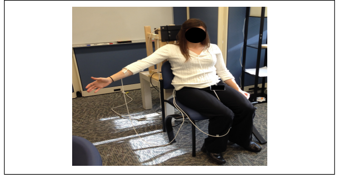
Figure 4: Subject positioning for motion analysis. Four sensors were attached to the subject and secured with a pre-wrap tape.
